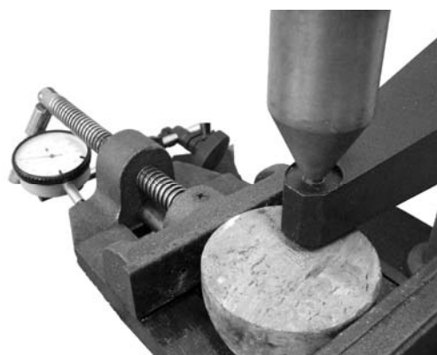
Figure 6 - Cerchar test apparatus
